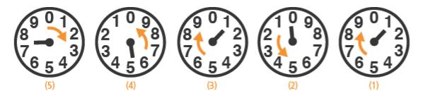
Some pointers move clockwise, others counter-clockwise. **Dials are read by starting at the right and moving to the left.** When a pointer is between two numbers, the smaller number is recorded.
