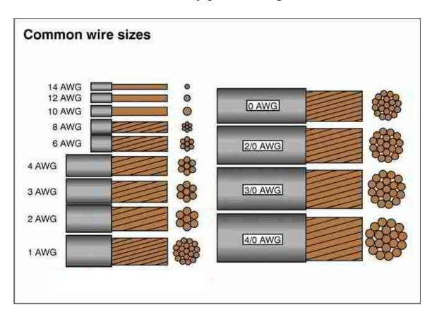
Electrical current is measured as ampacity. As a guide, #14 wire is good for \_\_\_\_ amps, #12 wire is good for \_\_\_\_ amps, #10 wire is good for \_\_\_\_ amps. As the number gets smaller, the size of the wire gets larger and the amount of amps it can handle also gets larger.
