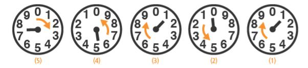
Some pointers move clockwise, others counter-clockwise. **Dials are read by starting at the right and moving to the left.** When a pointer is between two numbers, the smaller number is recorded.
