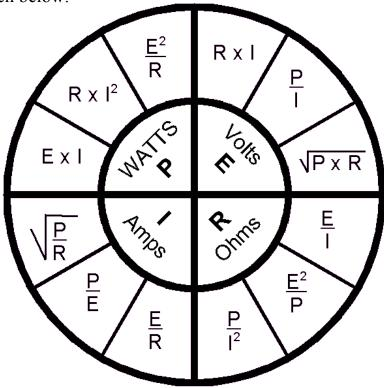
■ Example 1: Using the guide above, solve the following problem. A circuit has 60 volts and a resistance of 15 ohms. How many amps and watts are involved in this circuit?
