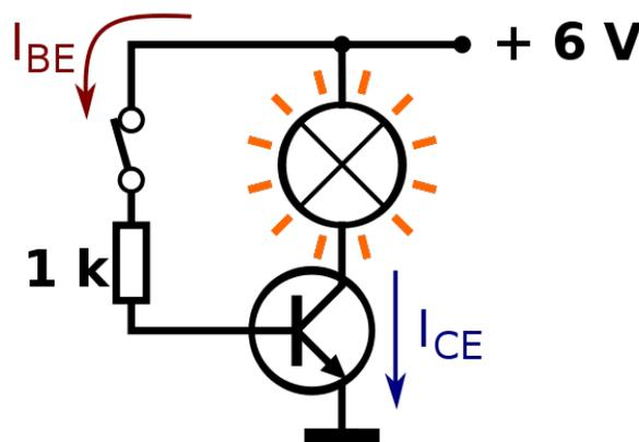
BJT used as an electronic switch, in grounded-emitter configuration. Transistors are commonly used in digital circuits as electronic switches which can be either in an "on" or "off" state, both for high-power applications such as switched-mode power supplies and for low-power applications such as logic gates. Important parameters for this application include the current switched, the voltage handled, and the switching speed, characterized by the rise and fall times.
