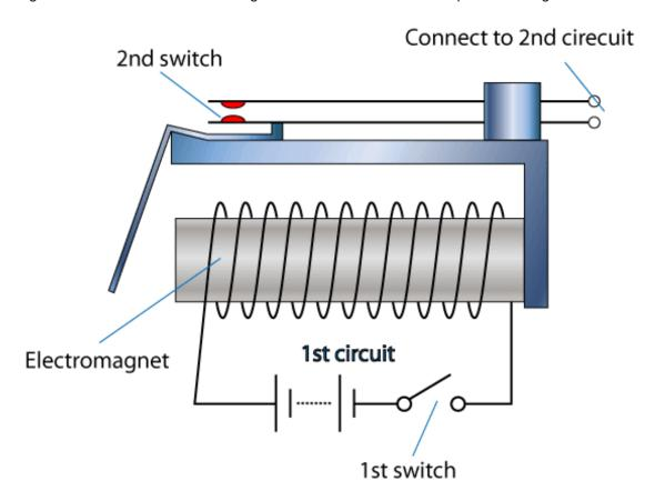
The main advantage of an electromagnet over a permanent magnet is that controlling the amount of electric current in the winding can quickly change the magnetic field. However, unlike a permanent magnet that needs no power, an electromagnet requires a continuous supply of current to maintain the magnetic field.
