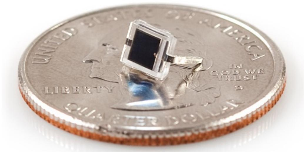
*A BPW34 photodiode (not the quarter, the little thing on top of that). Get it under the sun and it can generate about few  $\mu W$ 's of power!. Solar cells are the main benefactor of photodiode technology. But these diodes can also be used to detect light, or even communicate optically.*
